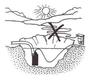
If the cable is very long, never wind it up in a roll, since this could lead to voltage loss.
