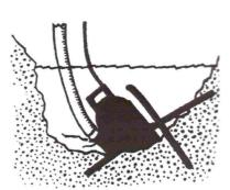
If the pump is to be placed in a stationary position and the medium to be conveyed is extremely soiled, it is recommendable to construct a sedimentation basin:
